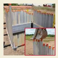
The Interlocking Aluminum Sheet Pile, designed solely for use with the Aluminum Sheeting Guide, is extruded from 6061-T6 Aluminum. Available in 13' sheet lengths, this strong, lightweight (48 lbs. per sheet) aluminum sheet pile also features a removable sheet driving cap.
